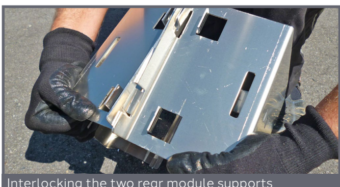
Interlocking the two rear module supports
