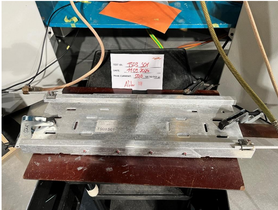
Figure 15: Test sample TS03 S01 after test with 3x 50 kA (10/350 µs).
