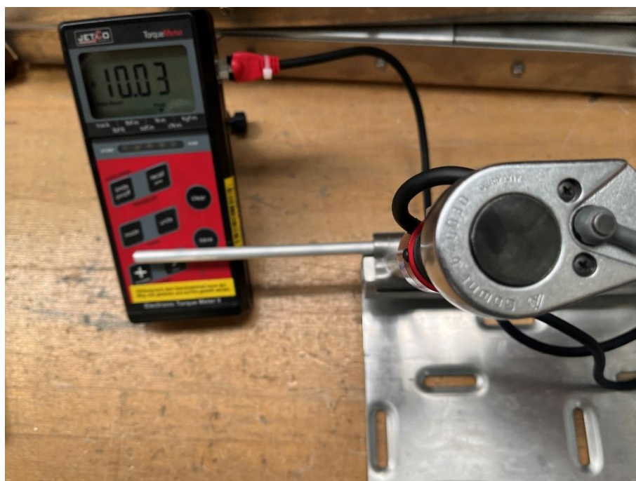
Figure 27: Measurement of torque – Uni – Earthingclamp 2.
