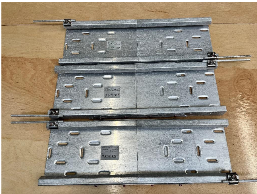
Figure 8: Test samples after the conditioning/ageing process.
