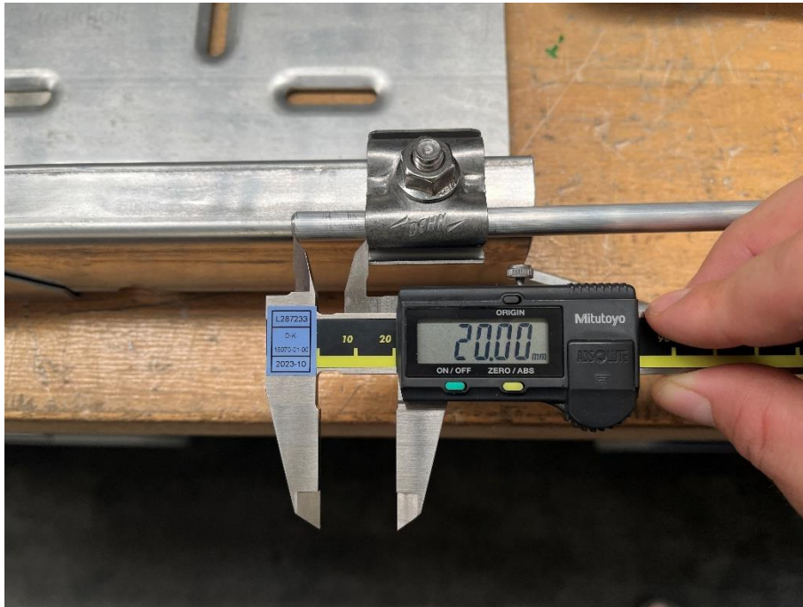
Figure 19: Measurement of conductor length after connector – Uni-Earthing Clamp 1.
