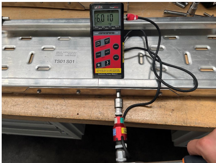
Figure 26: Measurement of torque – Self-drilling screw 2 – exemplary for self-drilling screws.
