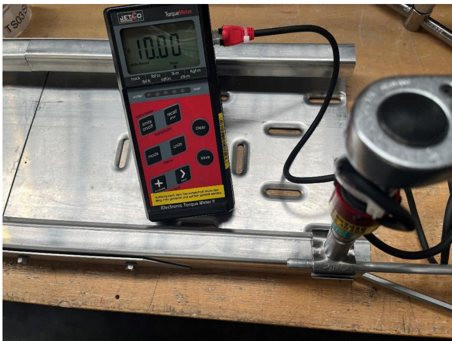
Figure 24: Measurement of torque – Uni – Earthingclamp 1.
