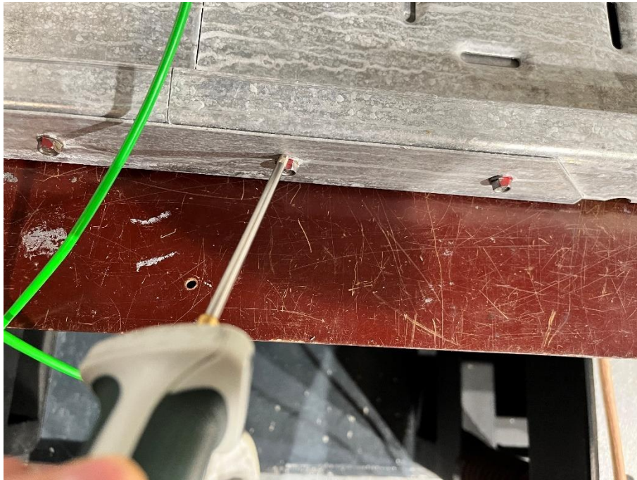
Figure 17: Measurement of test sample temperature – External connector.
